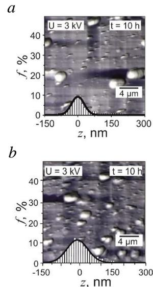
Fig. 1. SPM images of thin films of Al (a) and Al-1.5 at.% Fe alloy (b) deposited on glass substrate ( $U=3$  kV,  $t=6$  h) and the corresponding distribution histograms of heights of peaks and valleys of the surface nanorelief
