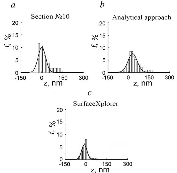
Fig. 3. Histograms of the distribution of heights of peaks and valleys of Al-1.5 at.% Fe alloy film ( $U=3$  kV,  $t=6$  h) shown in Fig. 2a: a – histogram of the roughness profile plotted along the scanning line No. 2, b and c - spatial nanorelief of the film surface with an area of  $20 \times 20 \mu\text{m}^2$ , determined using analytical processing of SPM data and application *SurfaceXplorer* software, respectively
