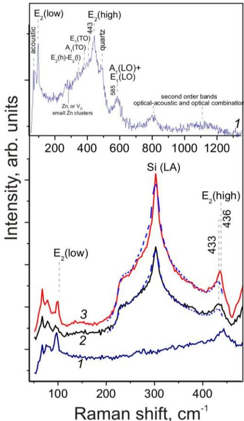
Fig.1. Raman spectra of ZnO (100 nm) films formed on quartz substrate (1) and on SiO<sub>2</sub>/Si substrate before (2) and after annealing (3). The dashed lines are corresponding normalized spectra of SiO<sub>2</sub>/Si substrate
