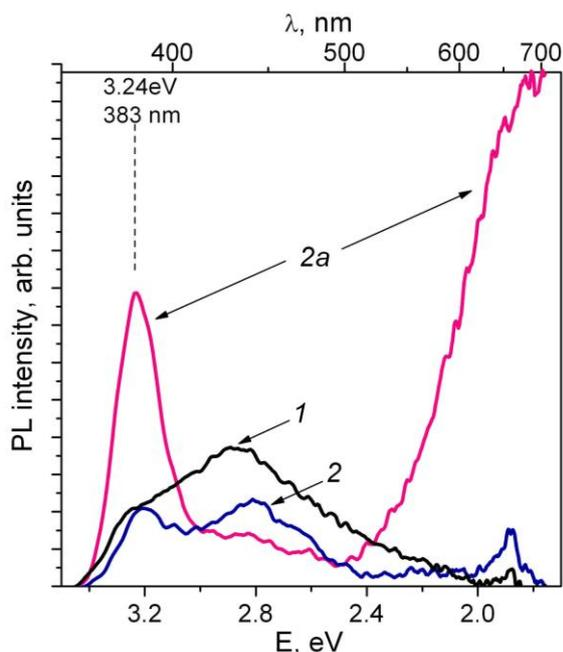
Fig. 5. PL spectra of annealed SiO<sub>2</sub>/Si substrate (1) and ZnO (100 nm) film deposited on SiO<sub>2</sub>/Si substrate before (2) and after annealing (2a)
