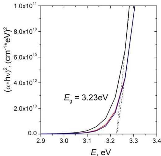
Fig. 3. Photon energy ( $E$ ) versus  $(\alpha E)^2$  for ZnO thin films with different thicknesses on quartz substrates
