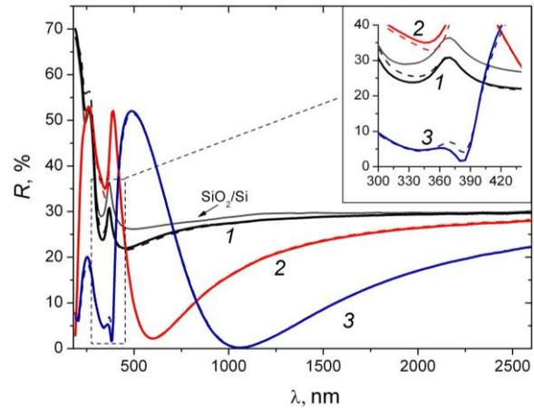
Fig. 4. Reflectance spectra of bare  $\text{SiO}_2/\text{Si}$  structure and ZnO films with thicknesses 14 (1), 40(2) and 100 nm (3) deposited on  $\text{SiO}_2/\text{Si}$  substrates before and after annealing (dashed lines)
