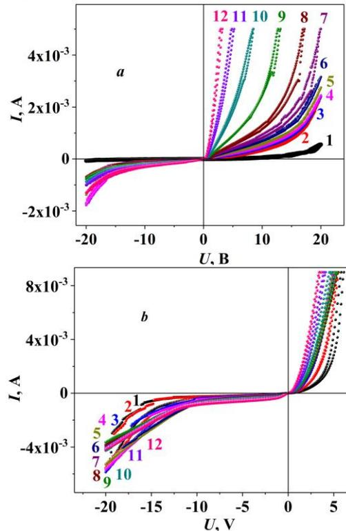
Fig. 1. I-V characteristics of the pristine (a) and annealed (b) samples at different temperatures  $T$ , K: 1 - 30; 2 - 50; 3 - 75; 4 - 100; 5 - 125; 6 - 150; 7 - 175; 8 - 200; 9 - 225; 10 - 250; 11 - 275; 12 - 300
