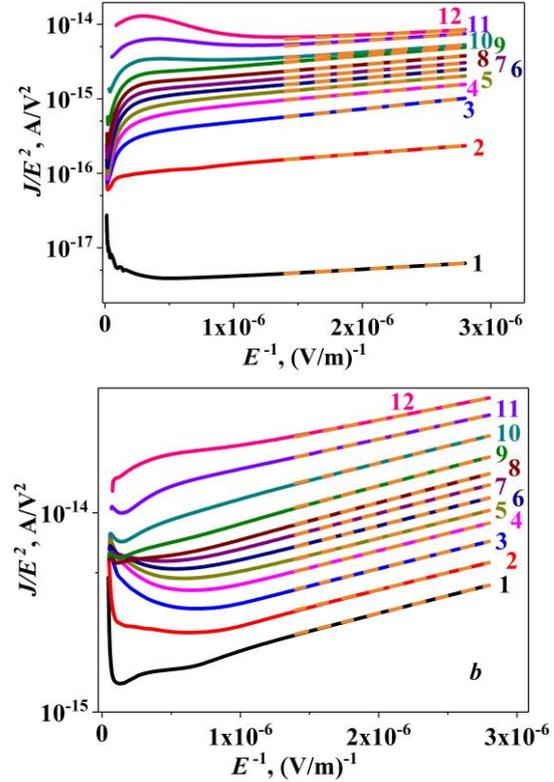
Fig. 3. Electric field dependences of the I–V characteristics of the initial (a) and annealed (b) samples at different temperatures  $T$ , K: 1 - 30; 2 - 50; 3 - 75; 4 - 100; 5 - 125; 6 - 150; 7 - 175; 8 - 200; 9 - 225; 10-250; 11 - 275; 12 - 300
