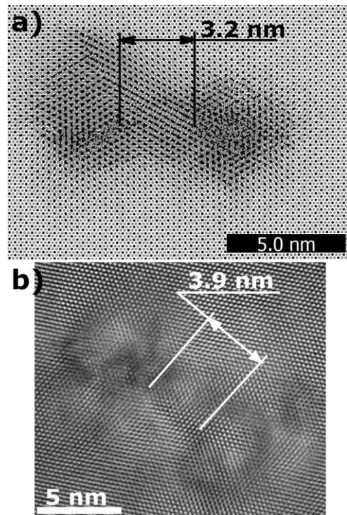
Fig. 1. (a) Results of a simulation of two subsequent impacts of Bi 700 MeV ions in  $\text{Al}_2\text{O}_3$  at 6.5 nm between trajectories. (b) TEM image of 700 MeV Bi ion tracks in  $\text{Al}_2\text{O}_3$
