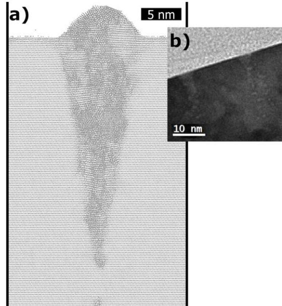
Fig. 3 (a) MD simulation of a 167 MeV Xe ion impact in  $Al_2O_3$  (2 nm slice of oxygen sublattice at 1 ns). (b) TEM image of conical tracks in  $Al_2O_3$
