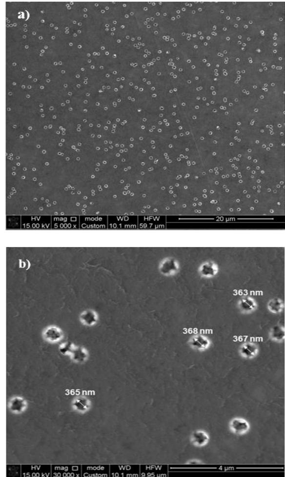
Fig. 1. SEM image of the surface after 30 minutes of chemical deposition: a) - total number of nanochannels, b) - nanochannel diameters
